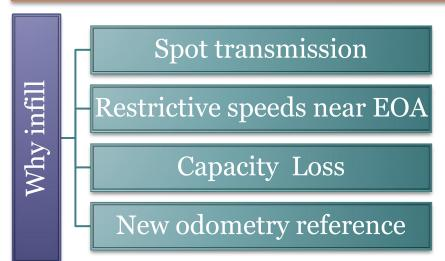
Primarily Balise based infill to be used. Optimum position for infill will depend upon traffic characteristic on the given line. An infill balise at 400-500m from signal provides a reasonable infill.
