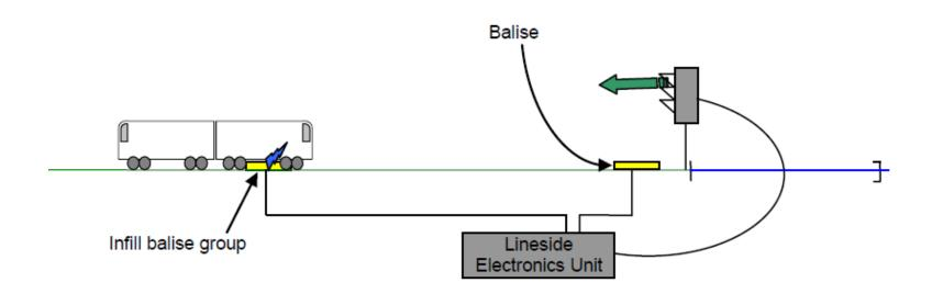
Release speed assists Infill function
